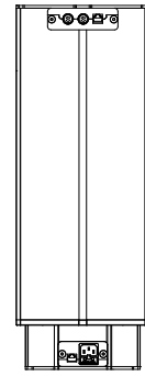
E = Tube: Thicker on top Sockets: Top side
