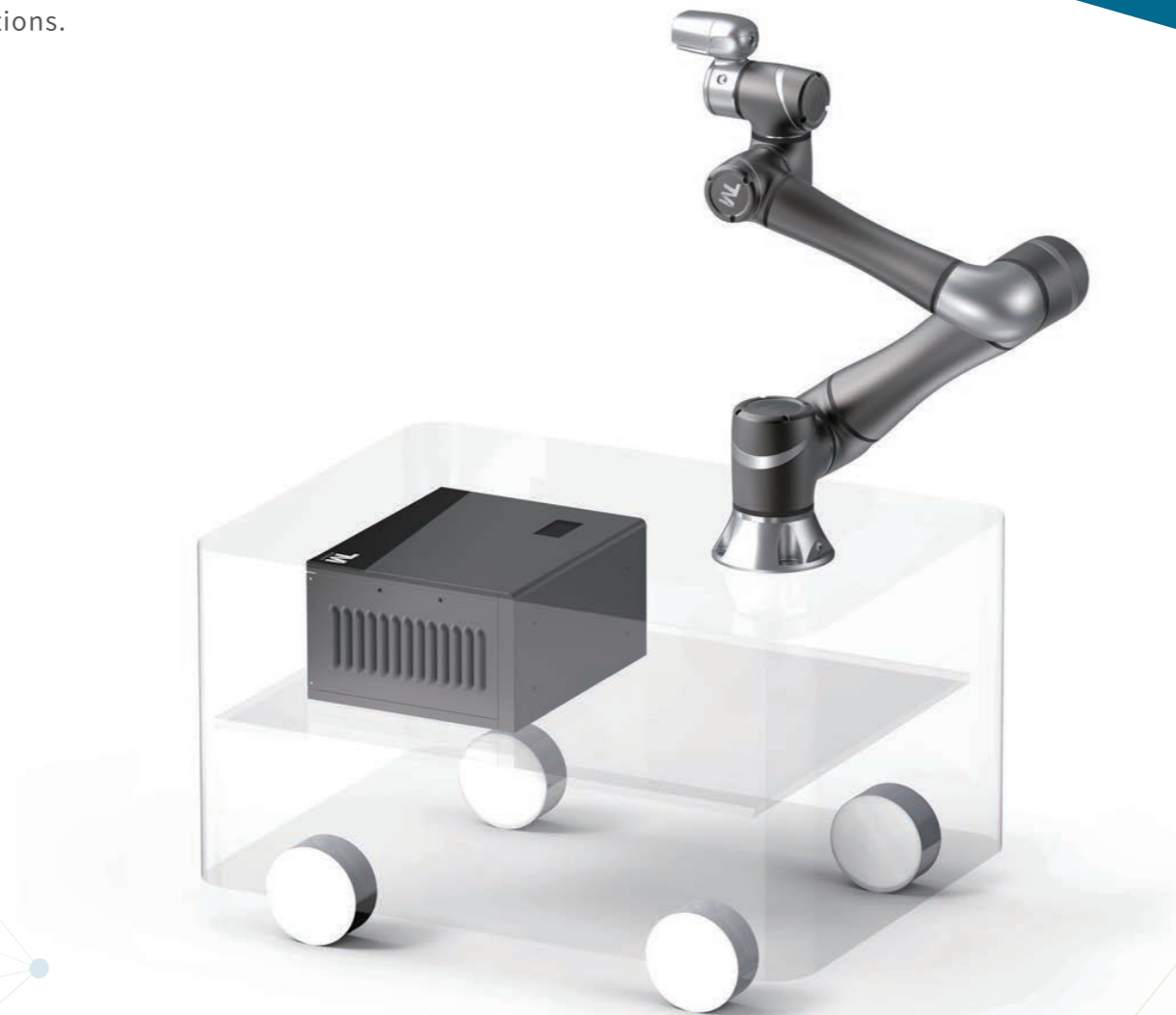
TM5M : Applicable for electronic industry mobile assembly.
