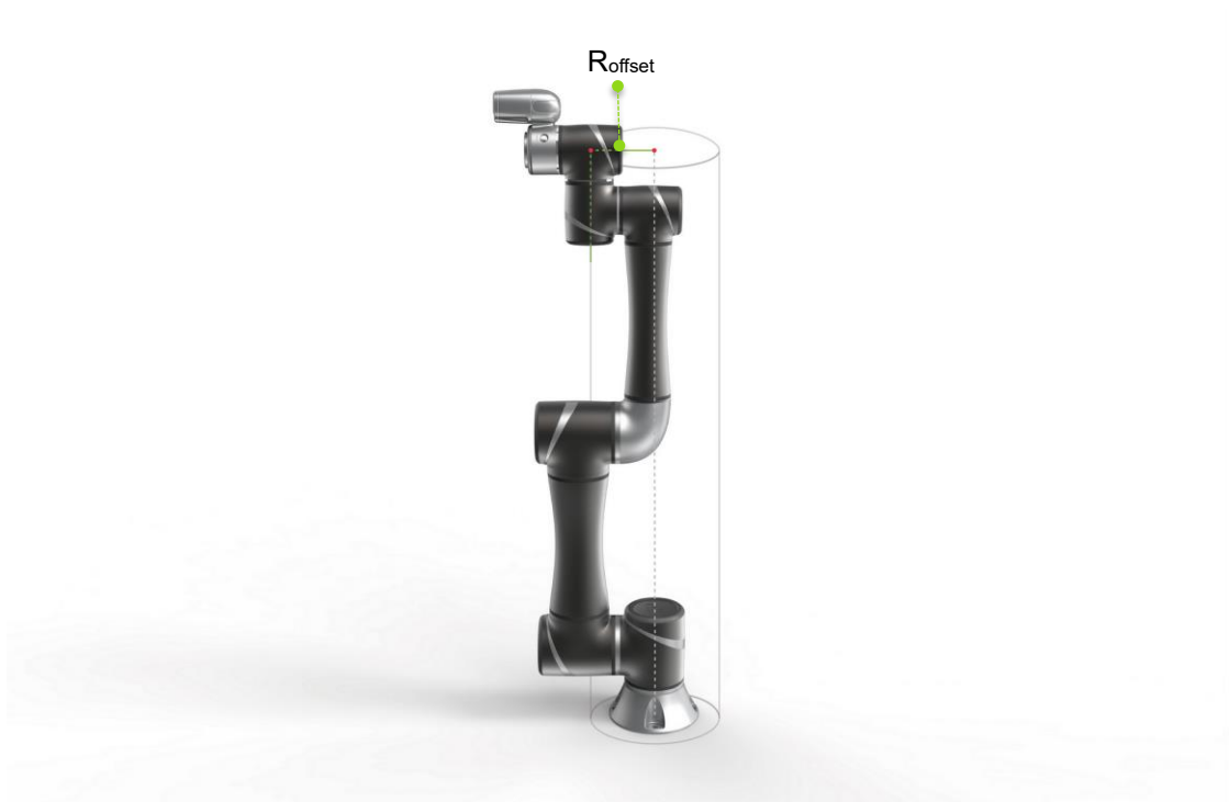
Figure 1: The Definition of R_{offset} .
