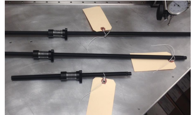
Far left: ATU Z axis actuator Second from left: Custom nut lead screw Right, top: Anti-backlash lead screw assemblies Right, bottom: Lead screw assembly
