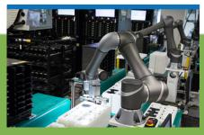
Using proprietary vision algorithms, the robot reads barcodes, locates trays of parts, and re-orients to a new workspace after being moved. The camera identifies precision points, eliminating the need for expensive fixtures or complicated operator routines to reorient the robot after moving, enabling quick redeployment.
