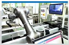
Automate your production without compromising on quality. Our cobots read bar codes, visually measure part features and stream data to other systems for traceability - to ensure production is accurate.
