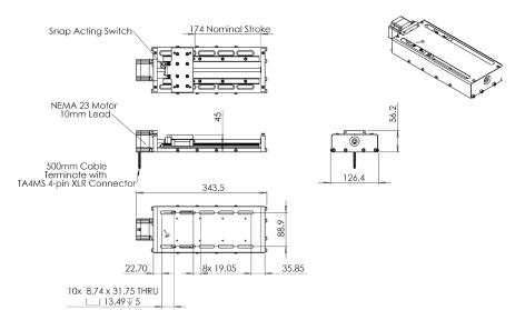
Integrated Stepper and Lead Screw Motor
