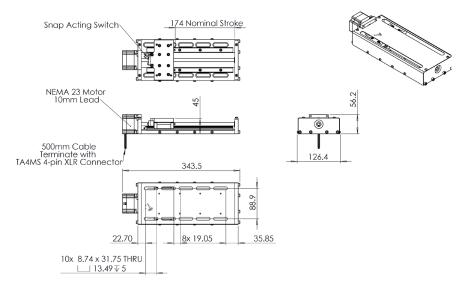
Integrated Stepper and Lead Screw Motor
