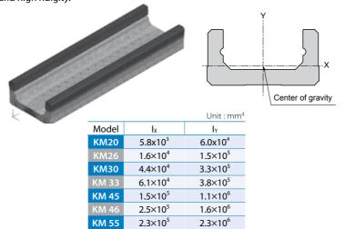
Note\* Ix: Geometrical moment of inertia around X axis Ω : Geometrical moment of inertia around Y axis
